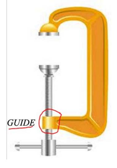
The helical (or helicoidal) guide ensures that the adjustable screw and cap(non removable link) move in a straight line. Since screw threads are needed inside the guide, it's why we call it helical.
